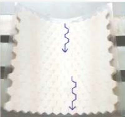
Path of the zigzag joint along the abrasive particles flow
