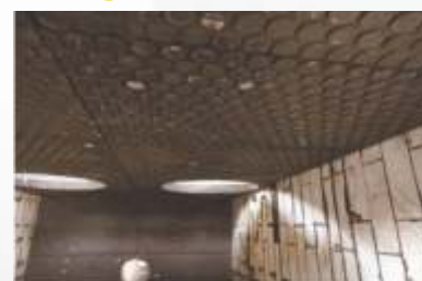
Rubber-ceramic plates with thickness 32 mm
